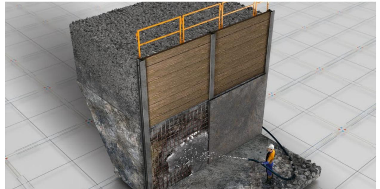
In discontinuous bored pile walls such as "king post" walls, bored piles incorporating vertical structural components (such as I-Beams, steel cages or precast elements) are installed with a greater gap. Shoring in the form of sheets, planks or shotcrete is subsequently placed between the structural elements during successive phases of the excavation process.
